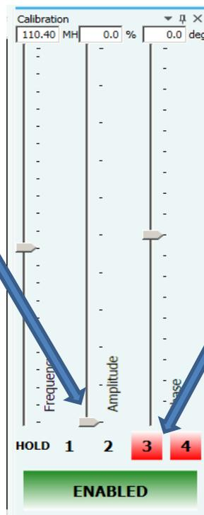
**Step 2:** Then select the HOLD button(s) under the channel(s) to turn OFF
