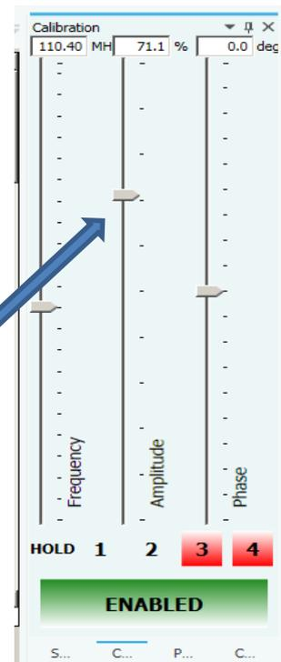
**Step 3:** Adjust the amplitude for the channels enabled (In this case Ch1 and Ch2)
